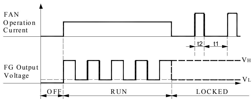
★Electrical Characteristics : ( at  $T_a = 25^\circ C$  ,  $Vcc = 12V$  )
