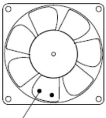
Note: The glues on the impeller
