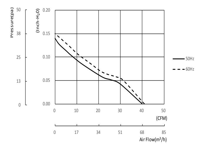
NOTE: The airflow and static pressure are measured with SUNON's specific fixture.
