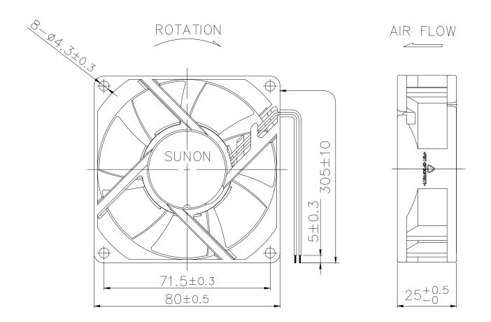
NOTE: 1.LEAD WIRE:UL3266 #24AWG GRAY 2.FRAME TYPE:FLANGE
