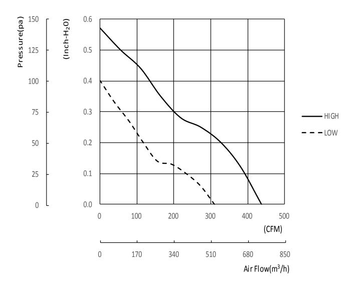
NOTE: The airflow and static press are measured with SUNON's specific fixture.
