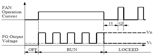
★Electrical Characteristics : (at  $Ta = 25^{\circ}C$ , Vcc = 12 Volt.)
