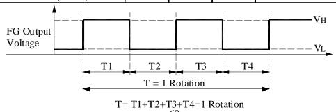
= T1+T2+T3+T4=1 Rotation  $T = \frac{60}{\text{rpm}}$
