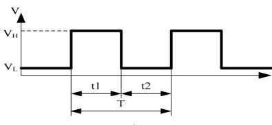
$$T = \frac{1}{f_{\text{PWM}}} = t1 + t2(\text{sec}) \quad . \label{eq:T_PWM}$$
