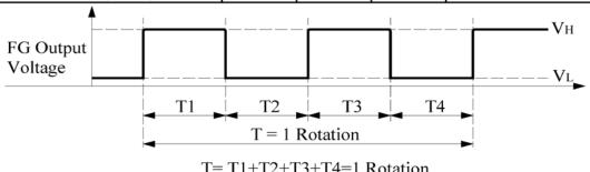
T=T1+T2+T3+T4=1 Rotation  $T=\frac{60}{\text{rpm}}$
