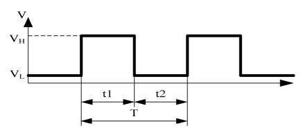
$$T = \frac{1}{f_{\text{PWM}}} = t1 + t2(sec) \quad . \label{eq:T_PWM}$$
