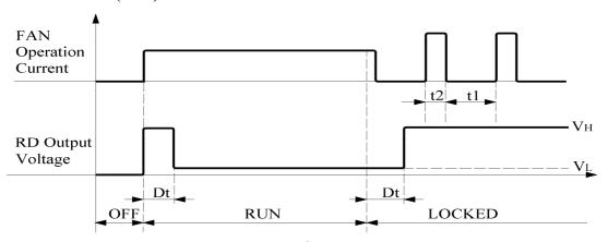
★Electrical Characteristics : (at  $Ta = 25^{\circ}C$ , Vcc = 48V)
