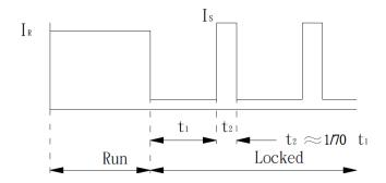
3rd wire signal Run : Square Wave Locked : Vmor VL
