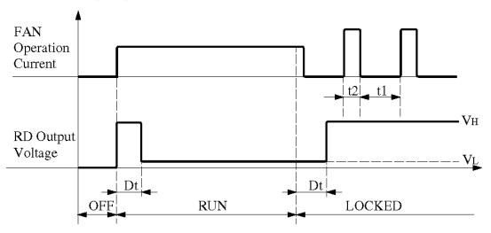
★Electrical Characteristics : (at  $Ta = 25^{\circ}$ C , Vcc = Rated Volt.)
