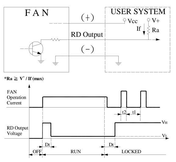
$\bigstar$  Electrical Characteristics : ( at Ta = 25°C , Vcc = Rated Volt.)
