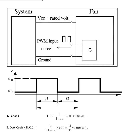
3.PWM Duty Cycle VS Speed ( Ta = 25°C, Vcc =Rated Volt., fpwm= 25 KHz)
