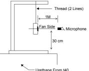
1 METER FROM MICROPHONE TO FAN INTAKE THE FAN IS RUNNING IN FREE AIR UNDER SHAFT HORIZONTAL CONDITION WITH THE MICROPHONE AT DISTANCE OF ONE METER FROM THE FAN INTAKE.
