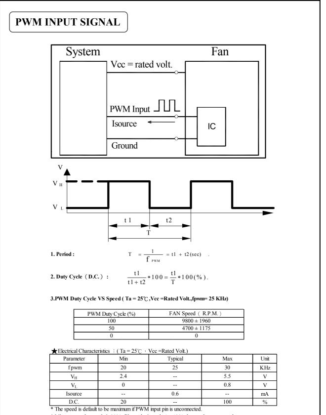
\* Min. start up duty cycle is 20% . Please don't apply  $1\sim19\%$  duty cycle to prevent the unstable fan speed.
