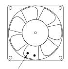
Note: The glues on the impeller is for impeller balance. Please don't remove it.
