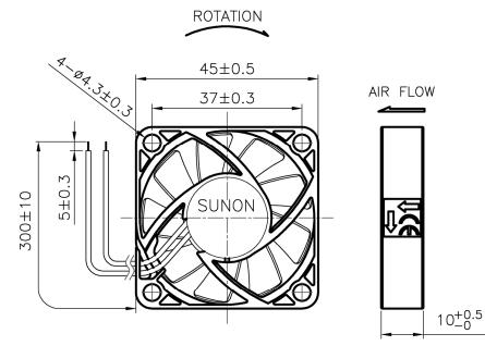
NOTE: 1.LEAD UL1007#26AWG RED WIRE----(+) BLACK WIRE----(-) 2.FRAME TYPE:RIB
