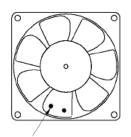
Note: The glues on the impeller is for impeller balance.
