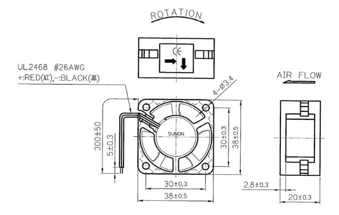
1.Air Flow Direction: Toward label side.2.Best Mounting Direction: Any orientation.
